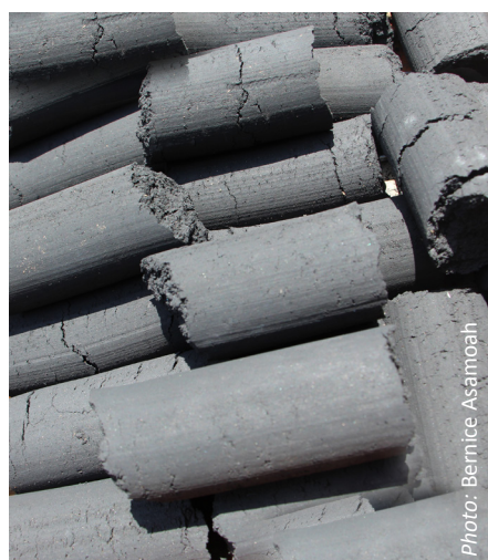
Typical briquettes produced by IWMI with locally collected solid waste.
